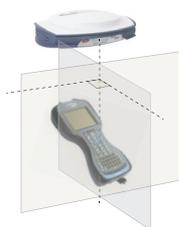
Making the pole vertical by reading the eLevel information displayed on the data collector screen will be more intuitive if you set up the rover as follows:
