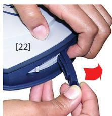
NOTE 1: If you only need to access the SD card holder, you may half-open the rubber flap. To do this, place three fingers on the area marked “SIM” on the flap while grasping the tongue to open the flap halfway (see [22]).
