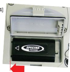
5. Close the trapdoor: It is good practice to use your two thumbs pushing thoroughly from the two corners of the trapdoor. By doing this, you will lock the snap-in hook properly and you will make the battery compartment fully waterproof.
