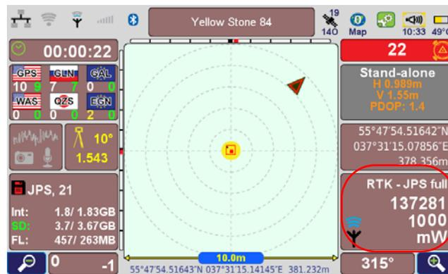
Figure 75. Base station is transmitting corrections
