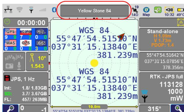
**Figure 43. Base station parameters**
