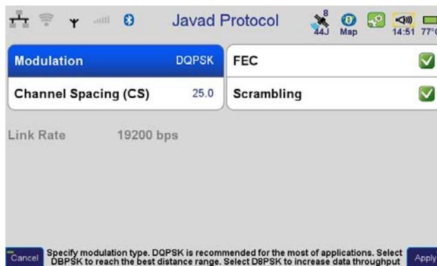
**Figure 63. Protocol parameters**
