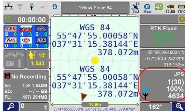
**Figure 85. Rover is receiving corrections**
