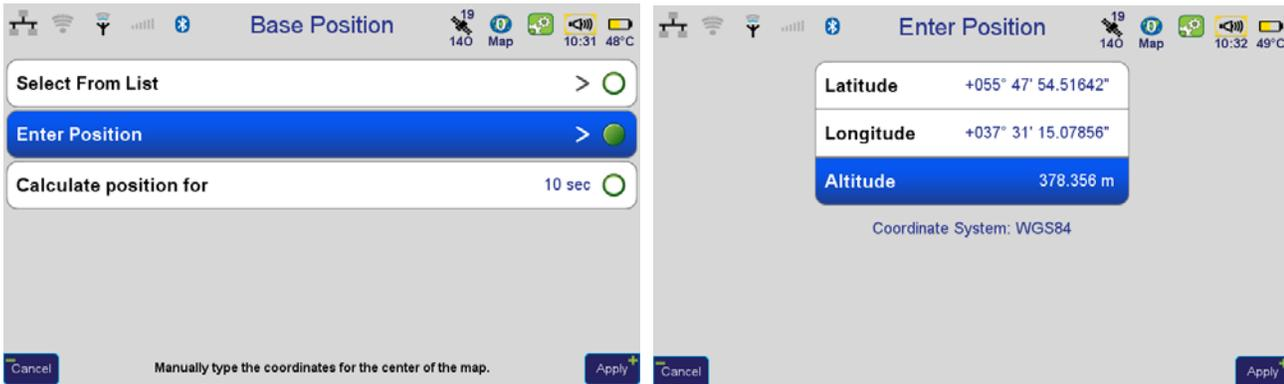
**Figure 44. Base station position**
