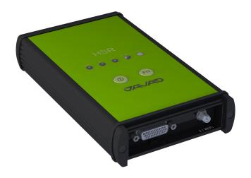
The new JAVAD High Speed Radio (HSR) utilizes unique Software-defined radio (SDR) architecture running on the powerful Xilinx System-on-a-Chip ZYNQ module in the conjunction with the high performance, highly integrated RF Agile Transceiver AD9361 from Analog Devices.
