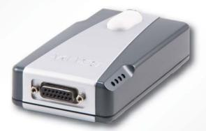
AW900BT radio transceiver is designed as universal license-free modem. It uses 902-928 MHz ISM (industrial, scientific and medical) license free USA band frequency hopping transmission techniques for excellent reliability in noisy plant environments and European CEPT license free 868-870 MHz band, allocated for narrow band telemetry, alarms and data transfer applications.
