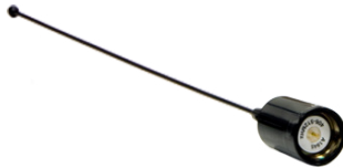
UHF NGP Antenna 406-430/430-450/ 450-470 MHz, 1/2, 2.4 dB gain, NMO p/n 30-587307-01 (optional)
