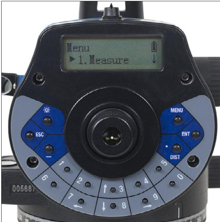
Figure 3.1 Control and display unit of the DL-15 digital level
