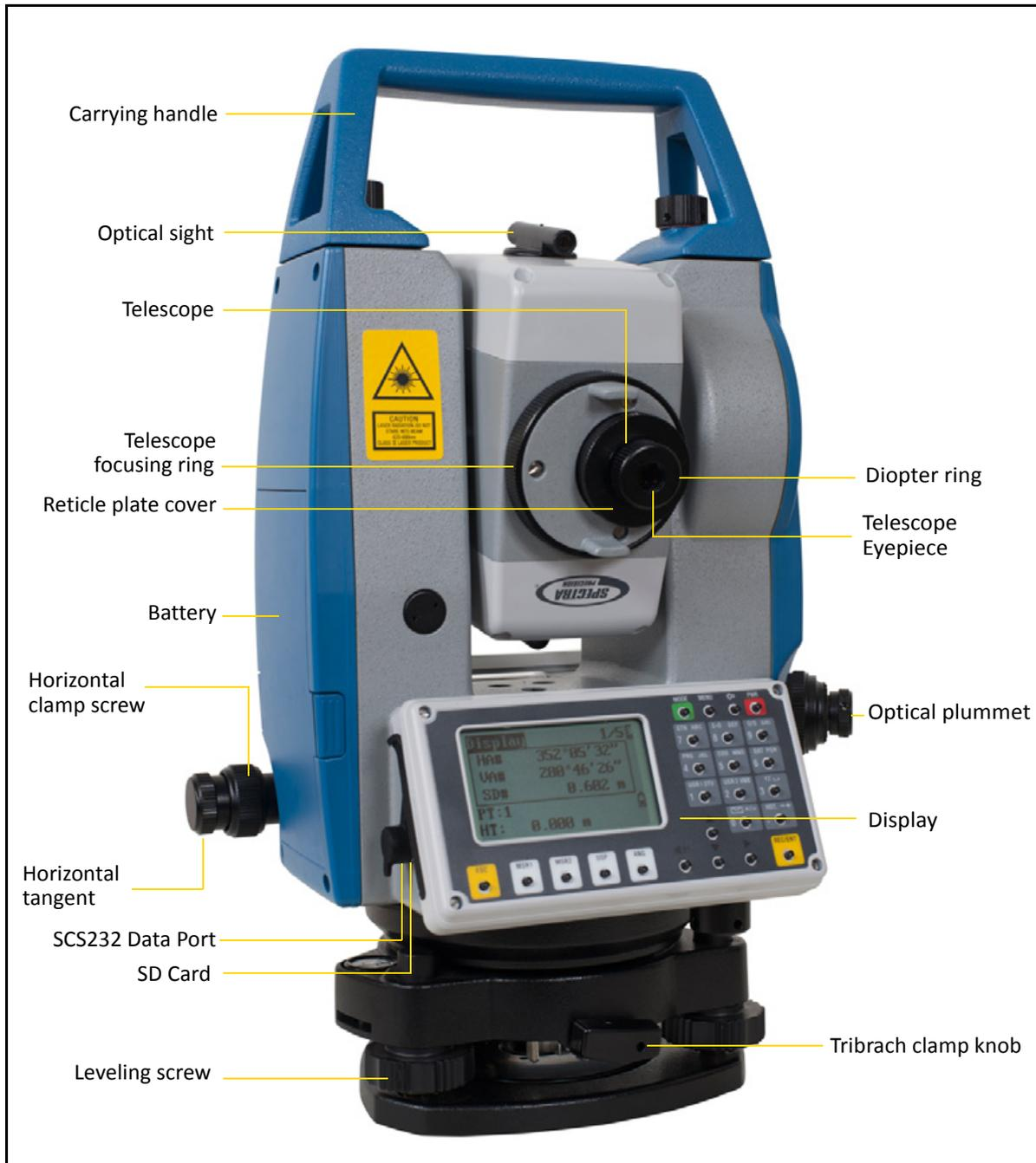
Figure 1.1 FOCUS 2 Series total station: Face 1
