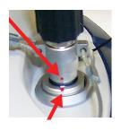
[9]: Power/data connector (DC input + RS232 serial port A). The connector socket is protected by a black rubber cap attached to the receiver case. Always keep the protection cap on when the connector is not used. This cap is a nonpolarized one.
