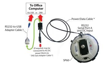
\*: All these items are part of the Office Power Kit P/N 94336 (option). Use the RS232-to-USB adapter cable if your computer is fitted with USB connectors (and no DB9 connector).
