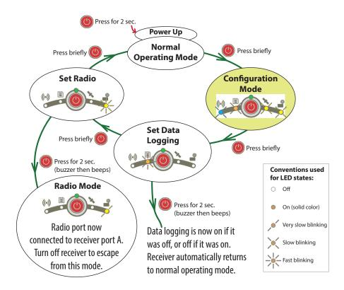
On the flowchart, each step is identified by a particular combination of LED states. Whatever the step, normal operating mode is restored after 10 seconds of user inactivity. NOTE: Other actions are possible from the control panel. See *Downloading Raw Data Files to a USB Key on page 37* and *Restoring Factory Settings on page 49*.
