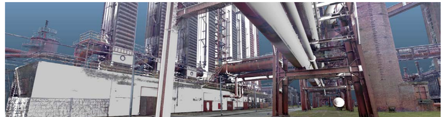
Point cloud with an overlaid CAD model, Zeche-Zollverein, Essen, Germany
